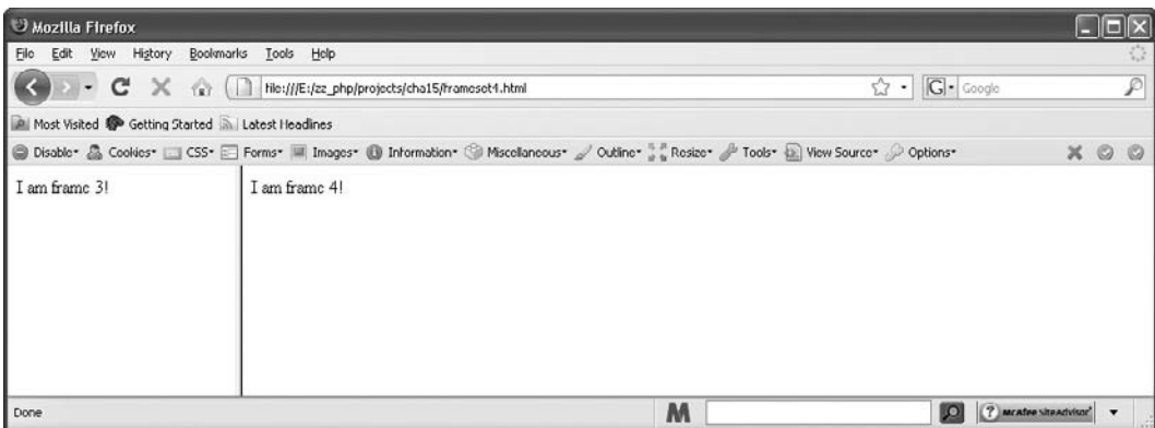
Figure 15-8 After the link is clicked, two new documents appear in the frames
